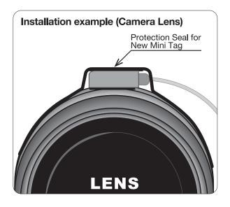
3. Remove backing paper of both sides of Protection Seal (B & C) and securely place on the merchandise.
