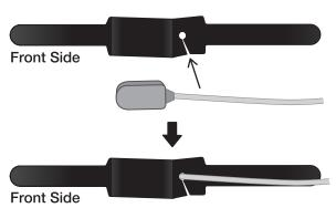
2. Remove backing paper on the center of Protection Seal (A) and securely install New Mini Tag.
